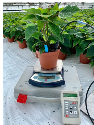
Figure 3. Plant-and-pot weights were measured with a portable electronic balance and a WET sensor was used to measure substrate VMC, pore E.C. and temperature. Photo taken on 3 September 2019.
