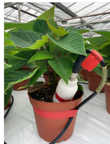
Figure 2. An SM150T moisture sensor positioned so that the measuring prongs provided an integrated measure of moisture content across the rooting zone. Photo taken on 3 September 2019.
