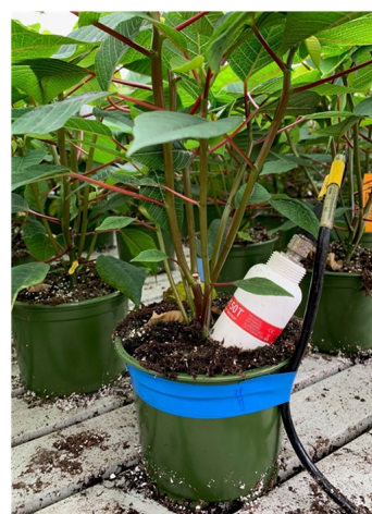
Figure 7. An SM150T substrate moisture sensor positioned so that the measuring prongs provide an integrated measure of moisture across the rooting zone. Photo taken on 24 September 2019.
