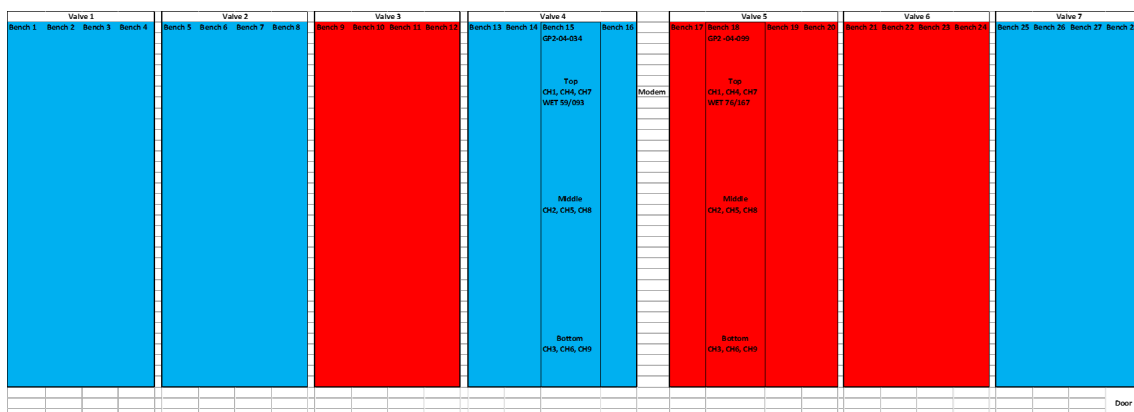
Figure 1. The experimental design for the RDI poinsettia experiment at Staplehurst Nurseries Ltd. Blue rectangles represent four benches in a CC irrigation block, red blocks indicate those allocated to the RDI treatment. The position of the nine moisture sensors sited across benches in blocks 4 and 5 is shown.
